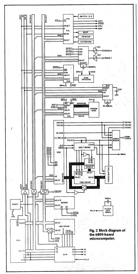
A battery backed-up real time clock and calendar. This is used by Flex to date stamp files. The clock chip also contains 50 bytes of nonvolatile RAM, some of which is used to maintain system parameters such as baud rates, floppy disc step rates, physical to logical mapping of disc drives and start-up parameters for the graphics device.
