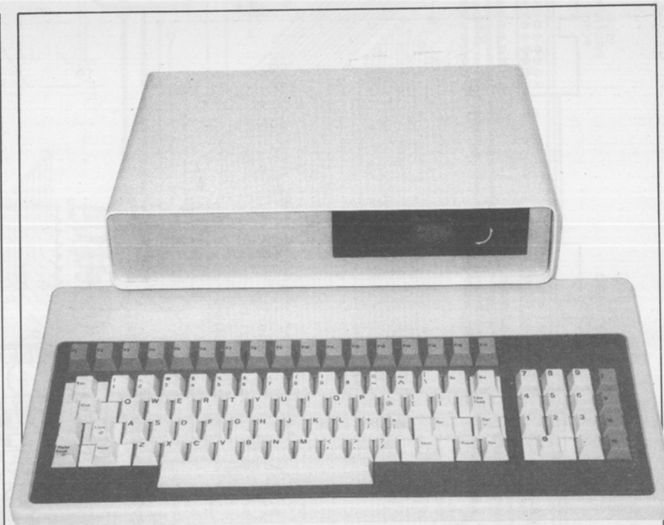
The 6809-based microcomputer fitted in a Vero case and equipped with a keyboard and 3.5" disc drive. Details of this and other case options will be given next month.
