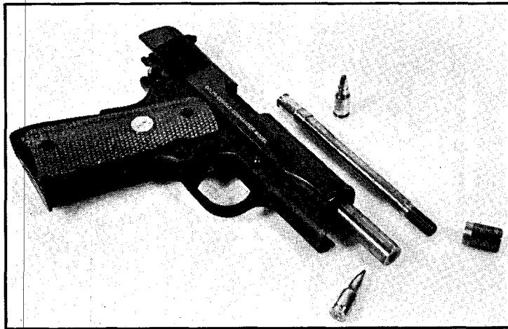
The initial attempt at chambering the .22 Super in a Commander was with a barrel insert held in place by a knurled nut. This was unsatisfactory, so Jim Boland lathe-turned and press-fit a new insert.
