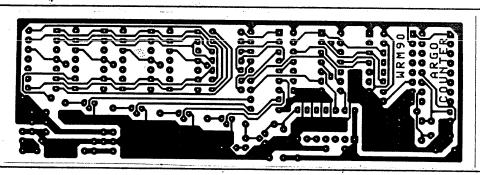
Unfortunately there was no component-overlay available when this newsletter went into production. For the experienced home-brewer, however, there should be no problems in placing the components correctly. The positions of the ICs are shown on the scheme to the right. R indicates the position of R4 to R10 (horizontally). The fat lines are wire links. An enlarged circuit diagram and/or a negative for the circuitboard can be obtained from the author or the editor.
